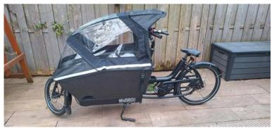
The Urban Arrow Family is an electric cargo bike with pedal assistance that can quickly and safely transport your children, pets and goods. The Urban Arrow cargo bike has a robust aluminum frame with an industrial-quality plastic cargo box, making it a very solid but also very light and agile cargo.
