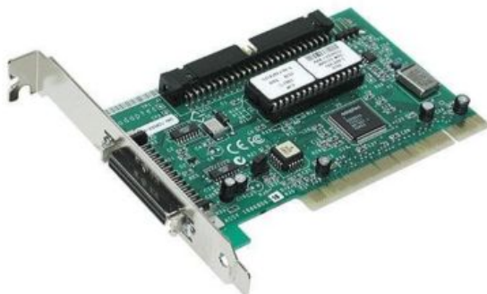
Internal 50-pin Standard (SCSI Male) connector
